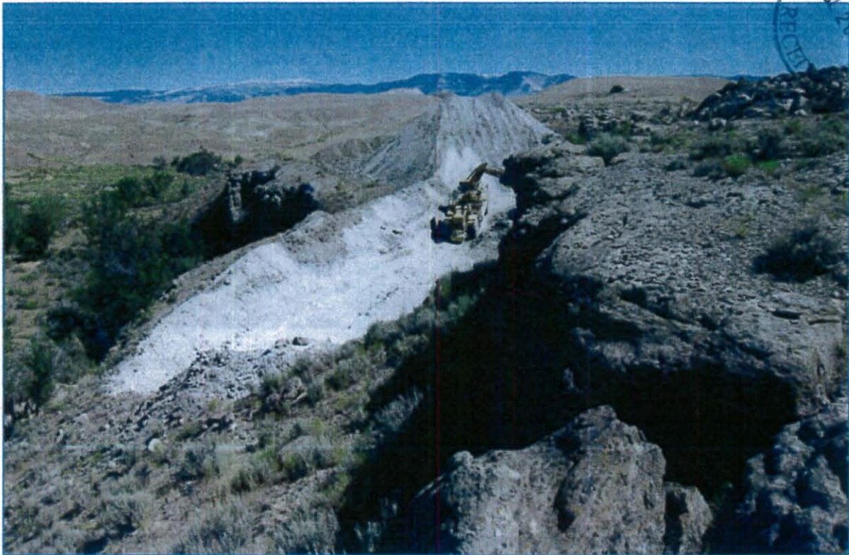
Photo 5 (above) looks to the north, showing the western edge of the active pit, with the trackhoe loading the Cat scraper. Overburden from the initial boxcut is shown in the background. Photo 6 (below) looks west along the haulroad that has been established along the Mi Swaco property boundary that connects the active pit area to the staging and pad areas.
