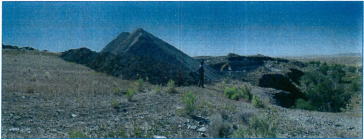
Photo 3 (above) looks southwest and shows the topsoil stockpile that has been constructed adjacent to the Access Road. Photo 4 (below) looks south at the active pit area (boom and bucket of the trackhoe are barely visible just to the right of photo center). Overburden from the initial boxcut has been stacked to the northeast. In the foreground is a windrow of what is construed to be suitable material.
