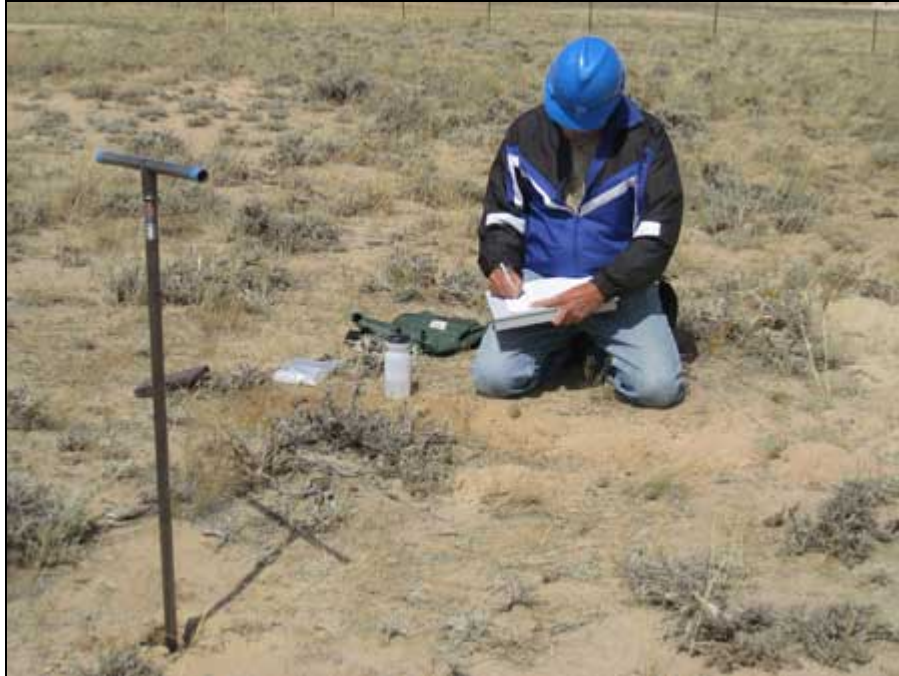
Mine Unit 1 Pit 10. Elevation 6968 ft. Vegetation on site had 60% ground cover, including 40% sage, 10% grasses & 10% lichens & other vegetation. Drilled to depth of 36 in.
