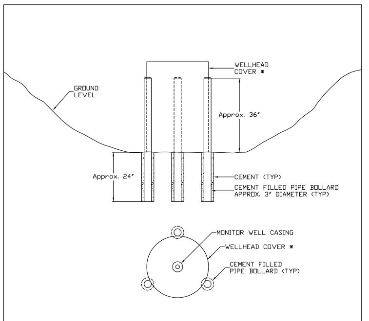
\* THE MATERIALS OF CONSTRUCTION WILL BE SUITABLE TO PROTECT AGAINST A TEN YEAR STORM EVENT (SUCH AS CULVERT, STEEL CASING, ETC.)
