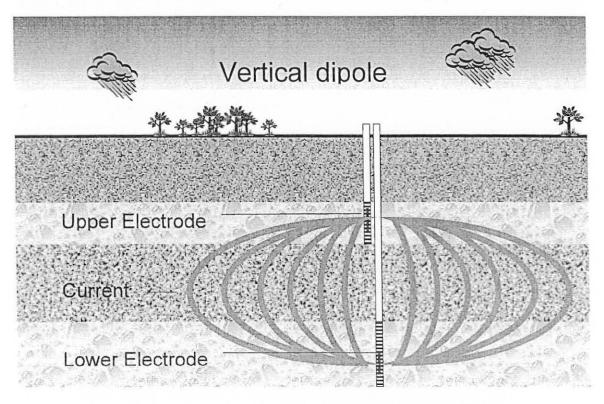
This flow pattern of electrical current will allow the upper or shallower groundwater, associated with R-8 well, to be identified and delineated. Because the electrical current concentrates in the upper water zone before bleeding off to the deeper electrode the effects of the magnetic signal near the surface of the ground can be detected and used to determine where electrical current is most present, thus identifying areas of high and low conductance in the shallow groundwater system.
