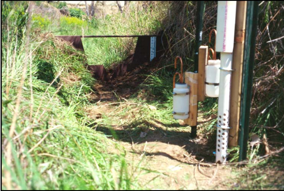
Figure 3.2-1. Partial Record station (Squaw Creek near Mouth) consisting of In Situ, Inc. Troll remote sampler housed in a perforated pipe, two-level single-stage water sampler array, and v-notch trapezoidal weir with staff gage.
